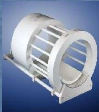
^1\text{H}/^{23}\text{Na} head coil for human imaging at 3 Tesla (Rapid, Würzburg).
